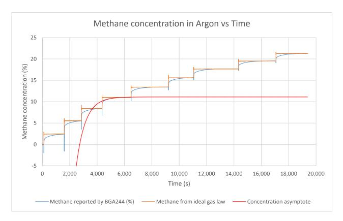
In the graph above, the methane concentration (computed from the temperature and pressure measurements and the ideal gas law) is shown in orange. The value reported by the BGA244 (showing the diffusion tails) is shown in blue. To estimate the asymptotic value of the concentration measurement, *A*, an equation was fit to each diffusion tail:
